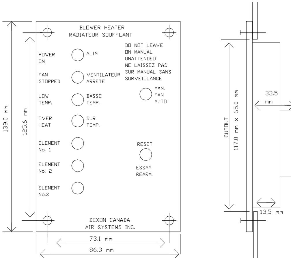
**The status board is not weather resistant and must be installed in an appropriate enclosure, remote from hazardous or corrosive locations in accordance with local electrical codes.**
