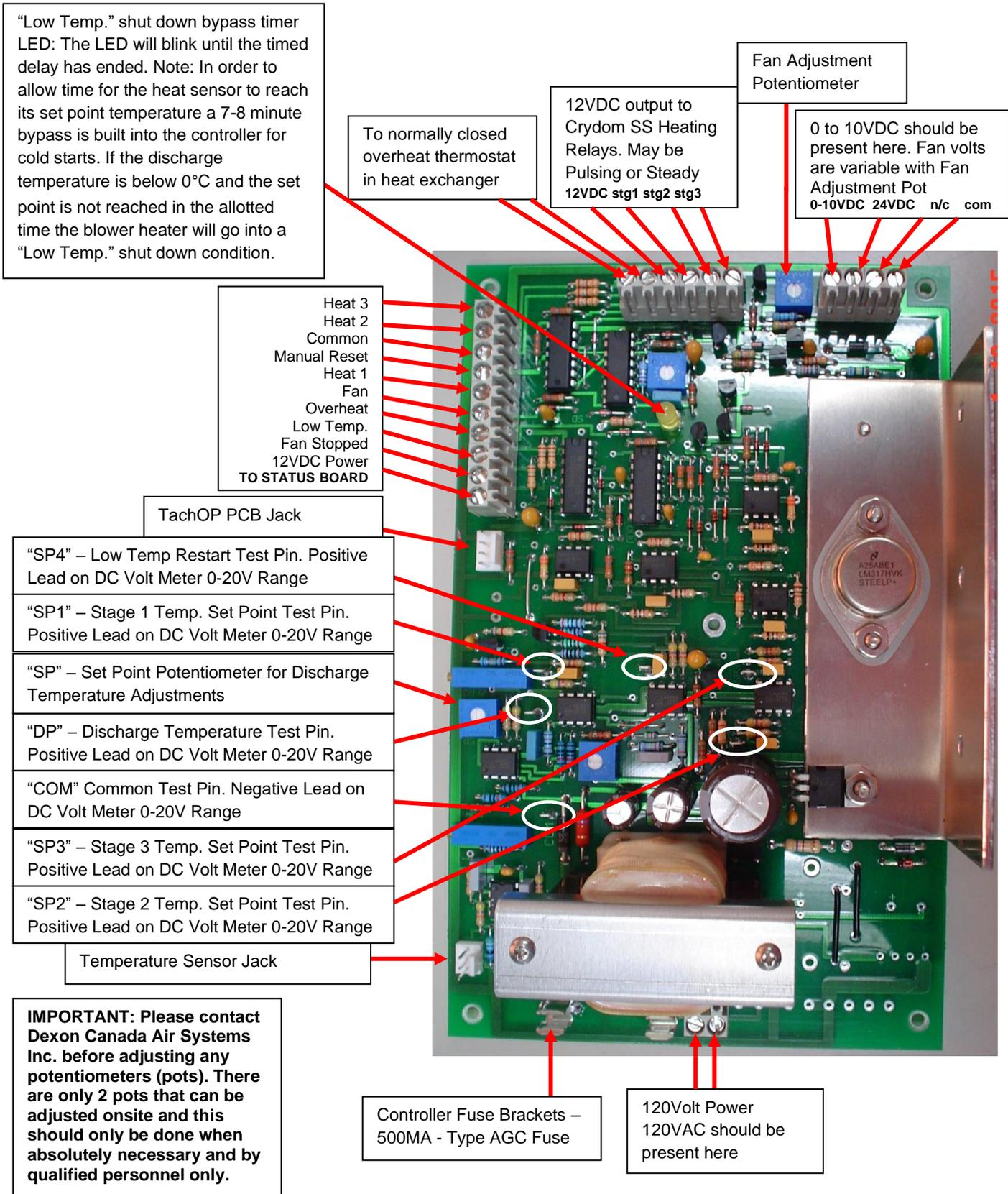
DEXON 95DH MAIN CONTROLLER TEST PINS DESCRIPTION
