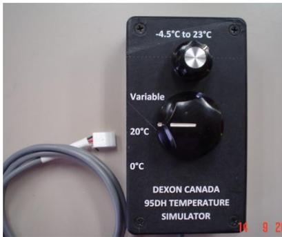
Fig. 2: Temperature Simulator
