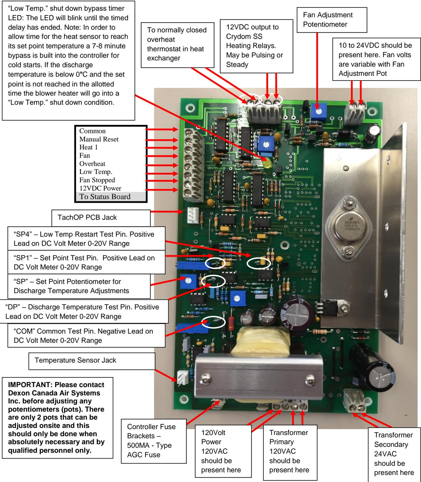
DEXON 95DH MAIN CONTROLLER TEST PINS DESCRIPTION
