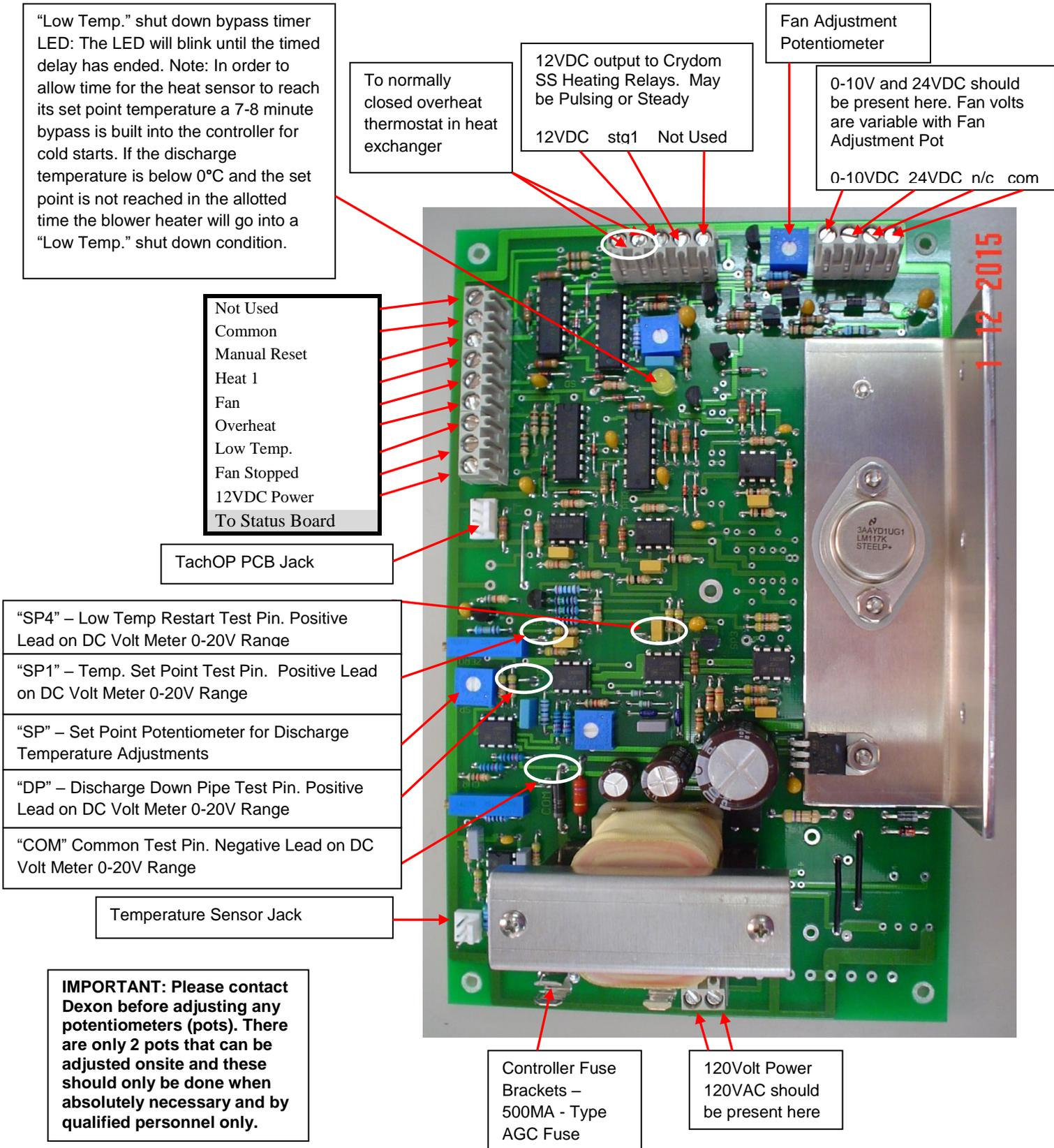
DEXON 95DH MAIN CONTROLLER TEST PINS DESCRIPTION
