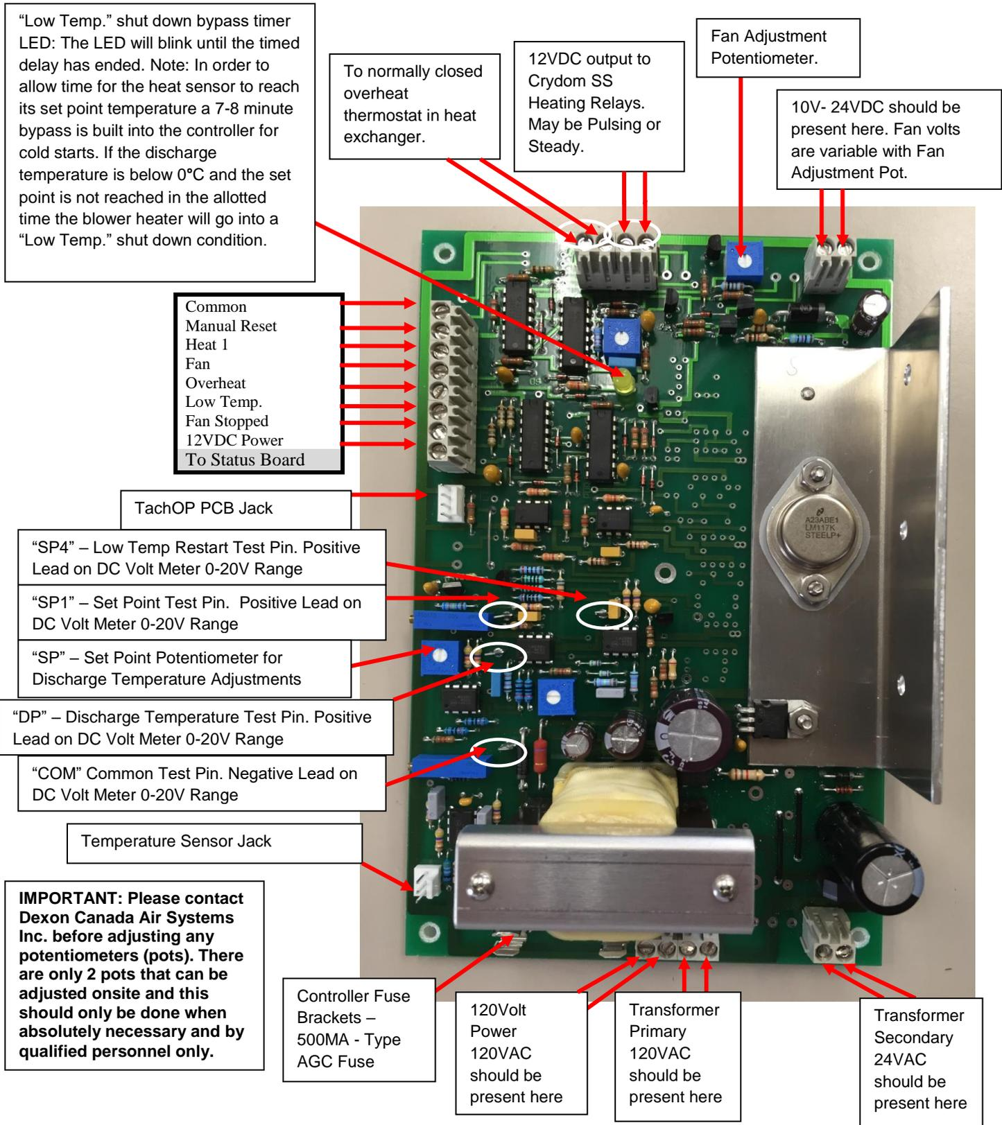
DEXON 95DH MAIN CONTROLLER TEST PINS DESCRIPTION
