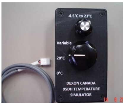
Fig. 2: RVDH Temperature Simulator
