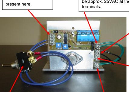
Transformer, secondary should be approx. 25VAC at these terminals.
