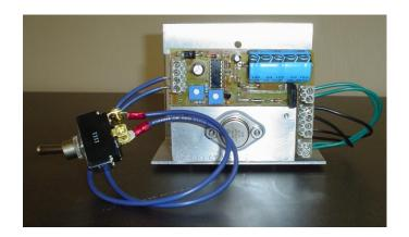
Power Supply/Speed Controller must be installed in appropriate enclosure remote from hazardous locations.
