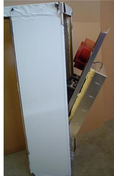
Fig.3 – To remove the control section pull top towards you (outward) and up off the 2 bottom pins
