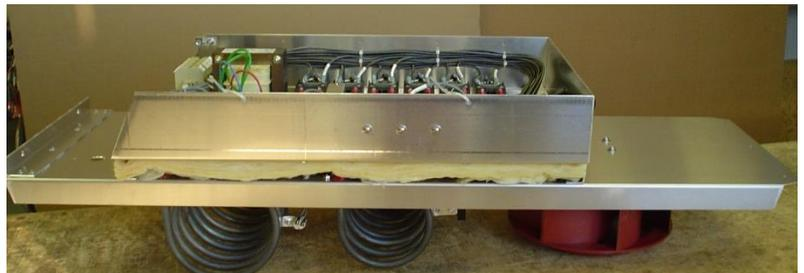
Fig. 4 – Once removed it can be inspected and repaired or shipped to Dexon. Must be shipped complete as shown. Do not separate panels when shipping to Dexon.
