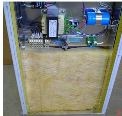
Fig.6 - When replacing the control section be sure to replace the insulation over the transition. Do not cover the electrical components.
