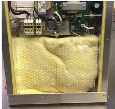
Fig.6- When replacing the control section be sure to replace the insulation on the transition only. Do not cover the electrical components
