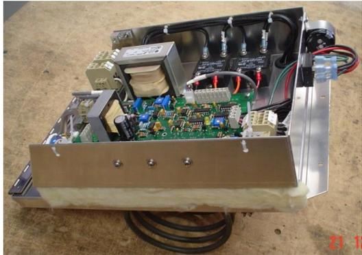
Fig. 4 - Once removed it can be inspected and repaired or shipped to Dexon. (Do not separate the panels when shipping to Dexon.) To access the fan you will need to remove 5 screws and the louver section from the top of the Blower Heater.
