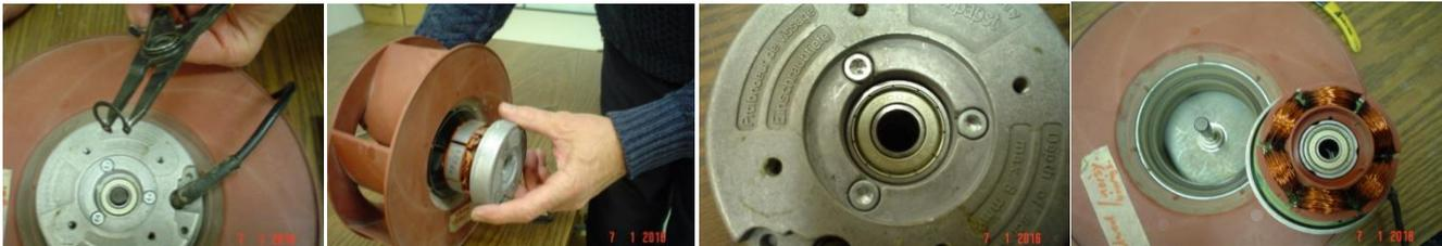
Pull the motor out from wheel (may be hard to pull apart). Bearings need to be changed on both sides. If the tension washers fall out, put them back in so they form tension against the bearing-opposing each other like this ).
