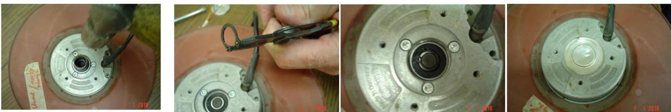
Gently tap the bearing into place with the piece of pipe and hammer. Please note the pipe should not rest on the bearing frame when you gently tap it as that might damage it. Replace the snap ring and using some type of adhesive put the cover back over the bearings.
