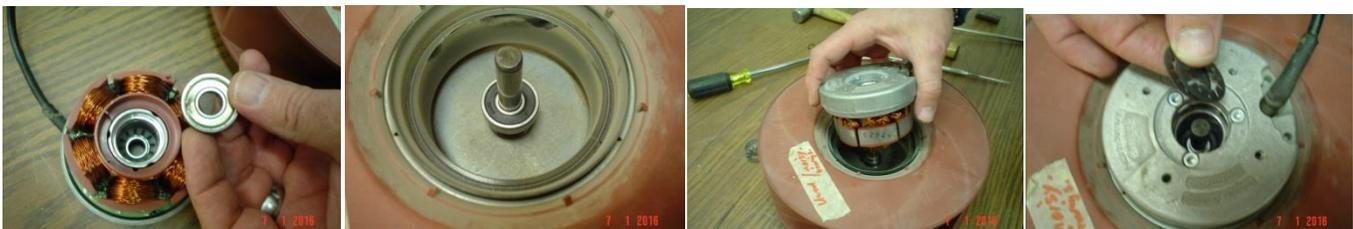
Put in the new bearings in place, easiest is to place the bearing on the shaft then placing the motor over the shaft and bearing. Make sure the spacers are still on the shaft before you put the second bearing on the motor
