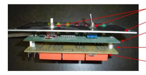
Toggle Switch and Reset Switch nuts
