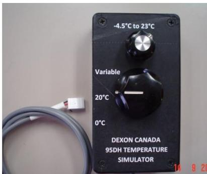
Fig. 2: Temperature Simulator
