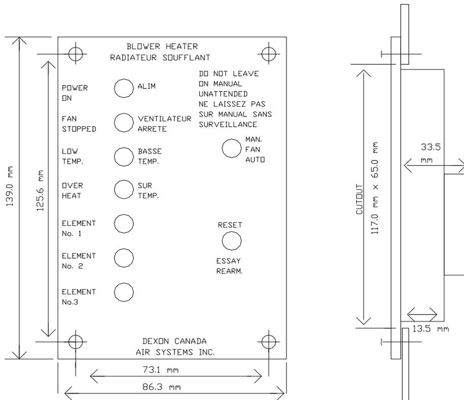
**The status board is not weather resistant and must be installed in an appropriate enclosure remote from hazardous or corrosive locations in accordance with local electrical codes.**
