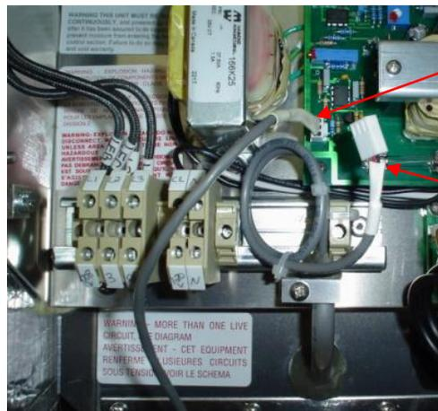
Temp. Sensor Jack with Dexon Simulator Connection
